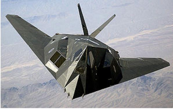
The F-117 (the logic behind its out-of-series designation still remains a bit mysterious) is a 'Stealth' attack aircraft. It uses a flat, angled fuselage and wing panels to direct radar reflections in a few sharply defined directions. Despite the
